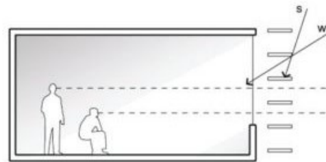
LOUVERS, blocks summer light and allows winter light while maintaining views
